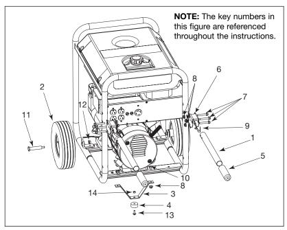
With the help of another person, tilt the generator and rest on frame as shown. DO NOT remove the shipping block until portability kit has been assembled.
